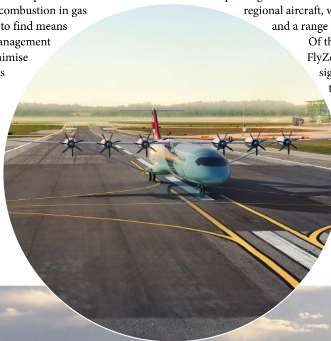
LEFT: THE REGIONAL CONCEPT BENCHMARKS THE ATR 72, AND IS INTENDED TO CARRY 75 PASSENGERS UP TO 800NM
